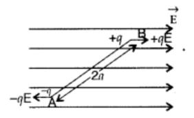
Hence, the net force acting on electric dipole held in a uniform electric field is zero.
